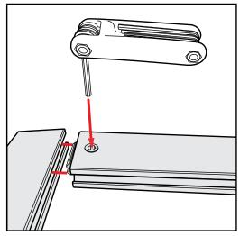
Extrusion & Lock Connection
