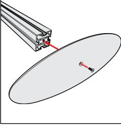
Base Plate & Extrusion Connection
